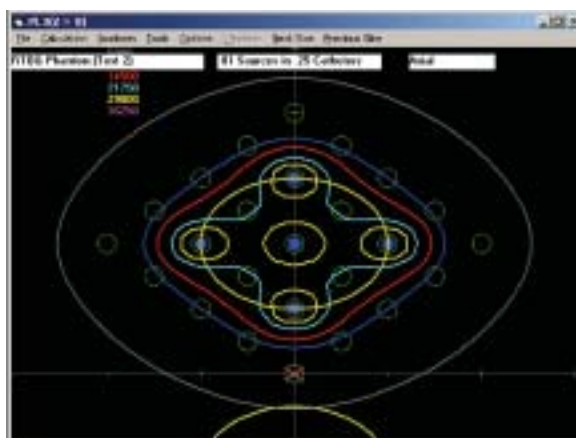
Figure 5c. The same slice with a 1-mm grid size. Note the marginal improvement over the 2-mm calculation grid.
